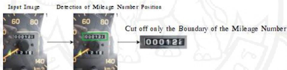
Figure 5 An example image of the result of the mileage's position detection procedure
