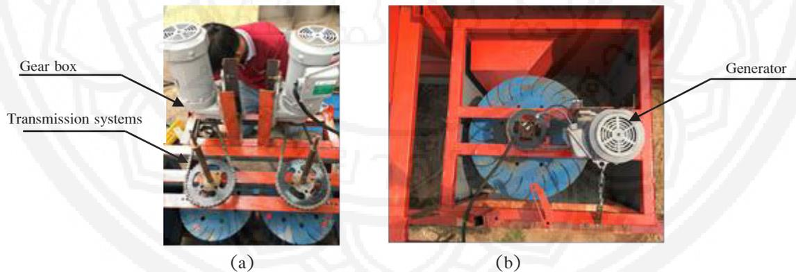
Figure 5 Installation of transmission and reduction system (a) dual-axis vertical turbine (b) single-axis vertical turbine
