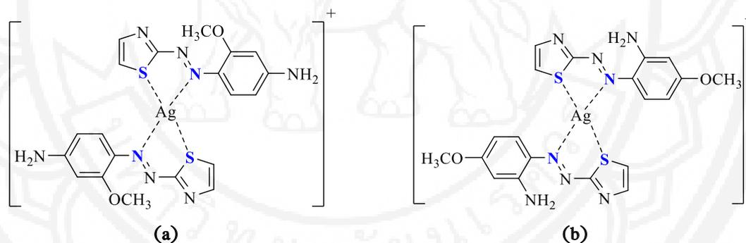
**Figure 2** Chemical structures of (a)  $\text{Ag(I)}-2-(2'-\text{thiazolylazo})-5\text{-aminoanisole}$  [ $\text{Ag}-(p\text{-TAAA})$ ] and (b)  $\text{Ag(I)}-4-(2'-\text{thiazolylazo})-3\text{-aminoanisole}$  [ $\text{Ag}-(o\text{-TAAA})$ ]
