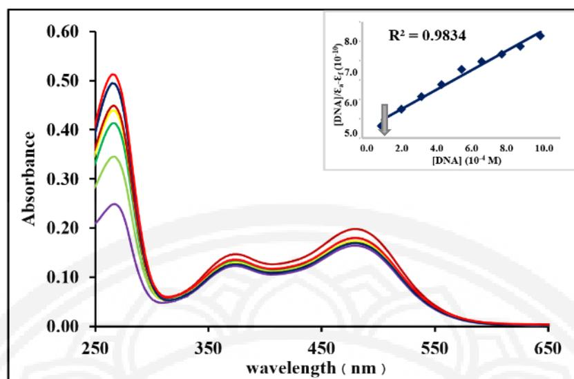
**Figure 7** Electronic absorption spectra of [Ag-(*o*-TAAA)] in the absence and presence of increasing amount of CT-DNA
