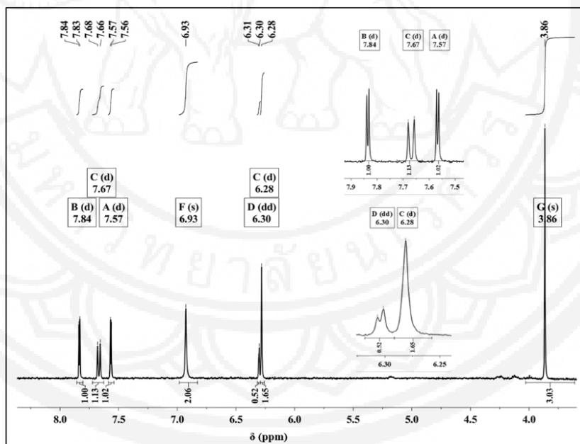
Figure 5 The  $^1\text{H}$  NMR spectrum of  $[\text{Ag}-(o\text{-TAAA})]$
