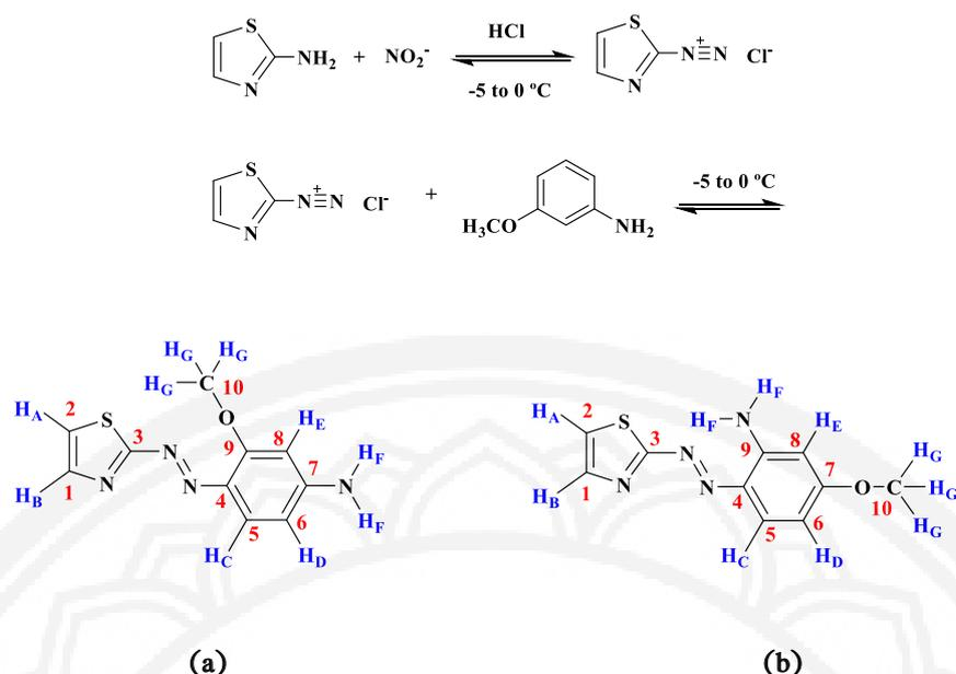
**Figure 1** Synthesis pathway and chemical structures of (a) 2-(2'-thiazolylazo)-5-aminoanisole (*p*-TAAA) and (b) 4-(2'-thiazolylazo)-3-aminoanisole (*o*-TAAA) with hydrogen and carbon atoms numbering
