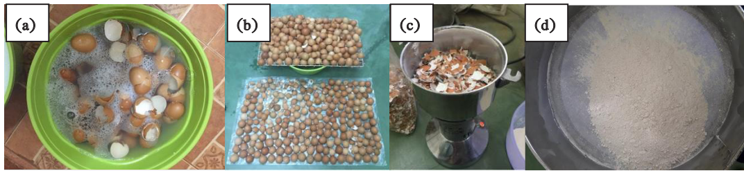
Figure 2 Steps for preparing chicken eggshells powder (a) cleaning (b) air-drying (c) grinding (d) sifting
