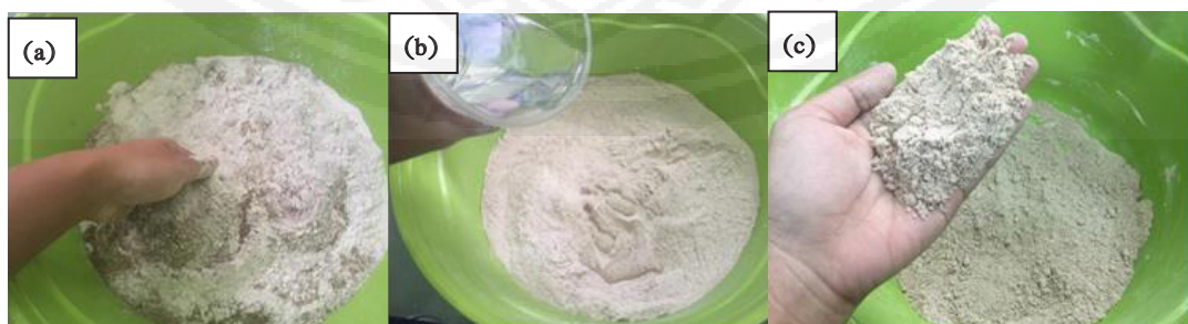
Figure 4 Steps for preparing mold material (a) mixing with bentonite (b) filling water (c) gently crumbling
