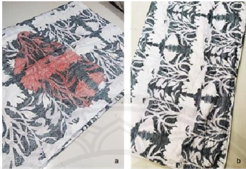
Figure 7 The example of results by using this developed blood stain remover with hospital's clothes after storing at room temperature in the 6 th month (a: before testing, b: after testing)
