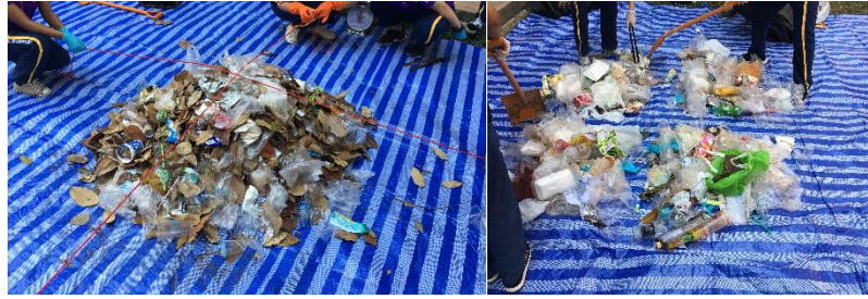
Figure 1 The figure shown represents the solid waste separated by using the quartering method
