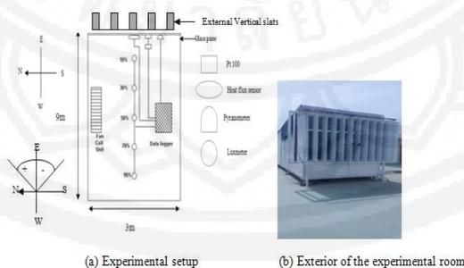
**Figure 1** Experimental room and setup
