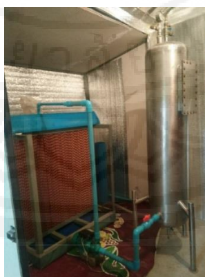
Figure 2 Experimental set up of the night cooling system
