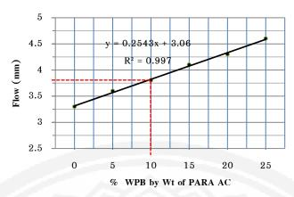
Figure 6 Flow values and quantity of plastic bag waste added to the para-asphalt concrete
