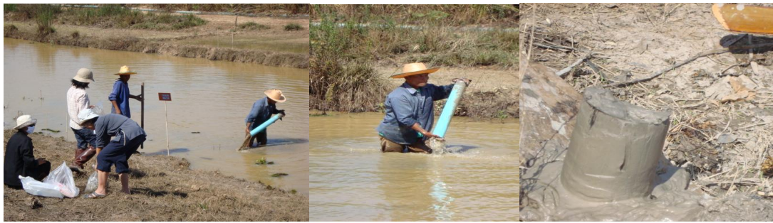
รูปที่ 3 Soil sampling by using a pvc pipe in the paddy fields before and after rice cultivation at Ban Bung Malaen Sawang Wirawong district, Ubon Ratchathani (in off-season rice year 2011)
