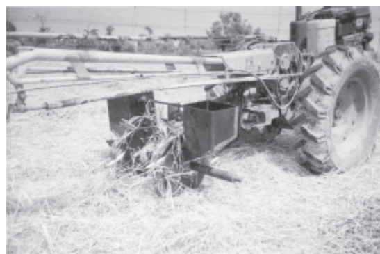
Figure 3. The rolling injection planter being tested in the field.
