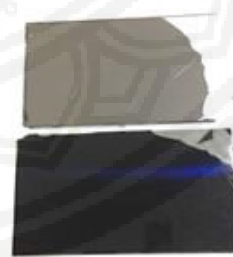
Figure 5 Two Pieces of iPad Screen, i.e., a Sepia Glass Plate / a Glass Plate with Black Film (Taken on 23 rd June 2019).
