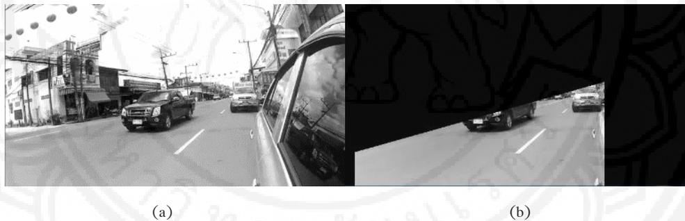
**Figure 9** (a) Output of gray scale module (b) Output of pre-processing image module
