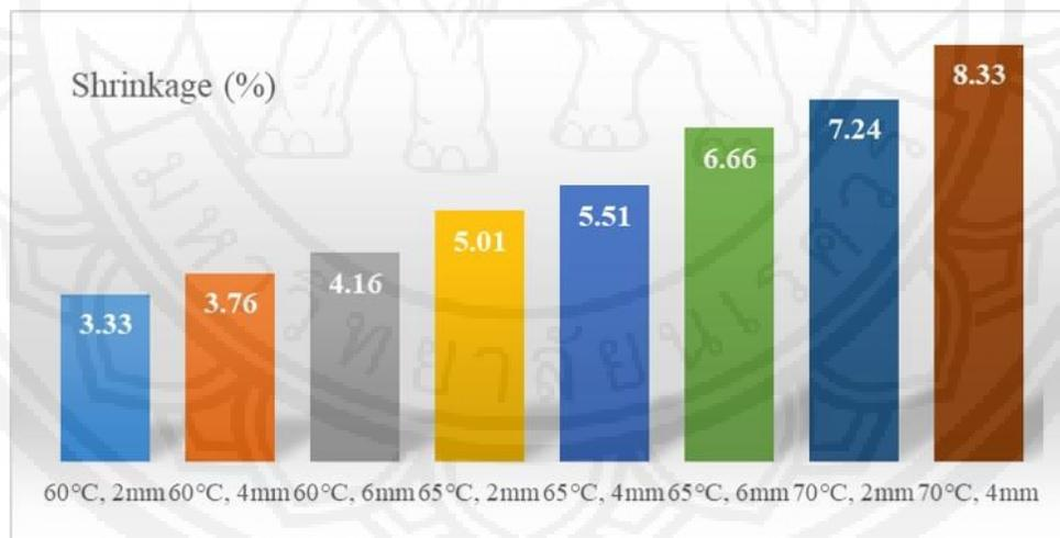
**Figure 4** Shrinkage of banana slices after drying each condition
