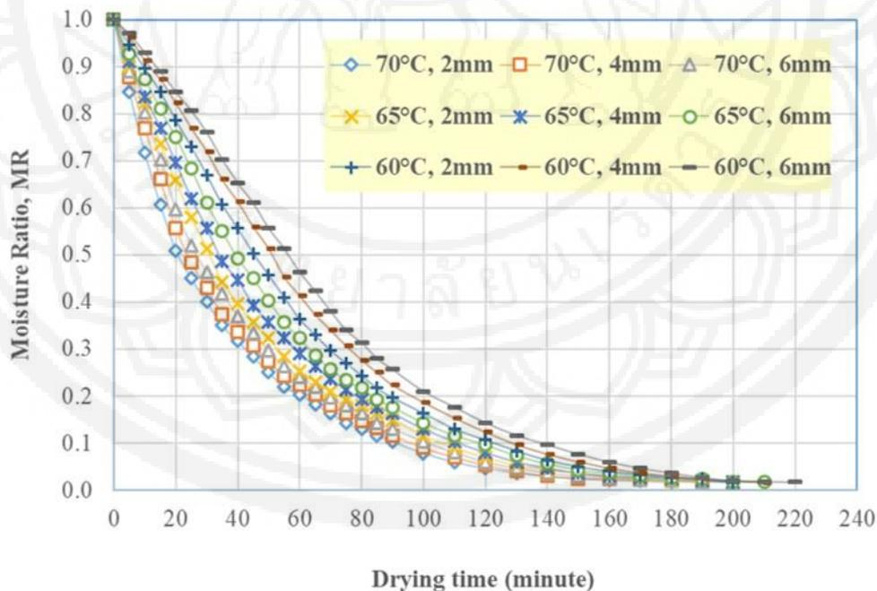
**Figure 3** The experimental results of banana slices with nine conditions
