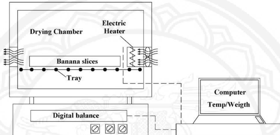
Figure 2 Schematic diagram of apparatus using hot air technique
