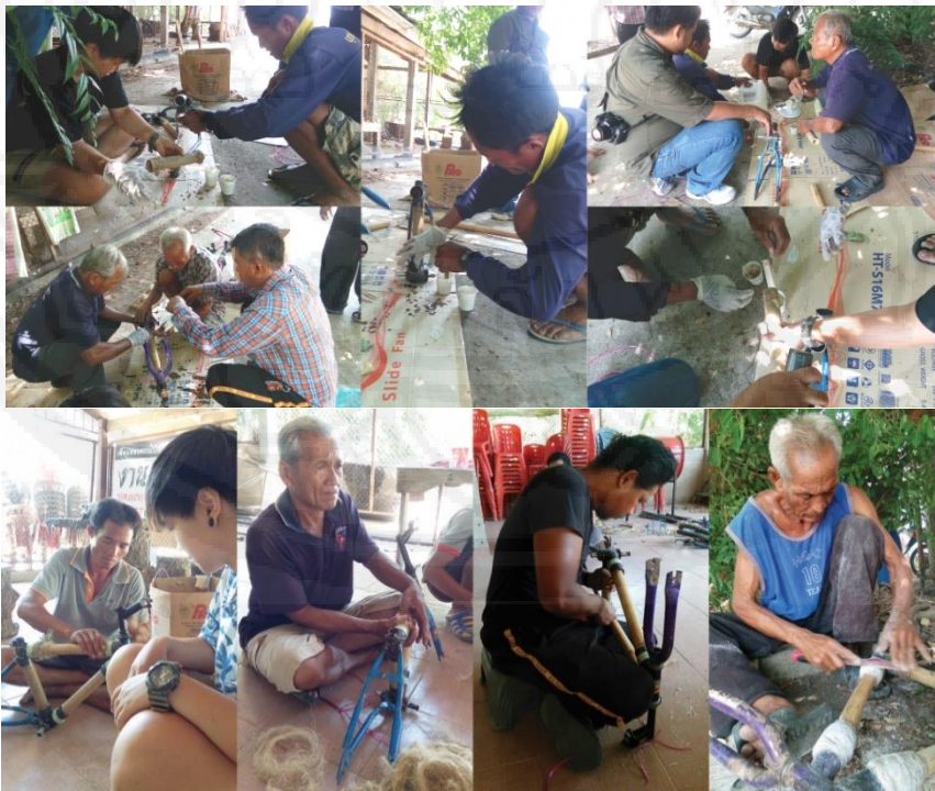
Figure 3 A demonstration of production processes of bamboo bikes by the community
